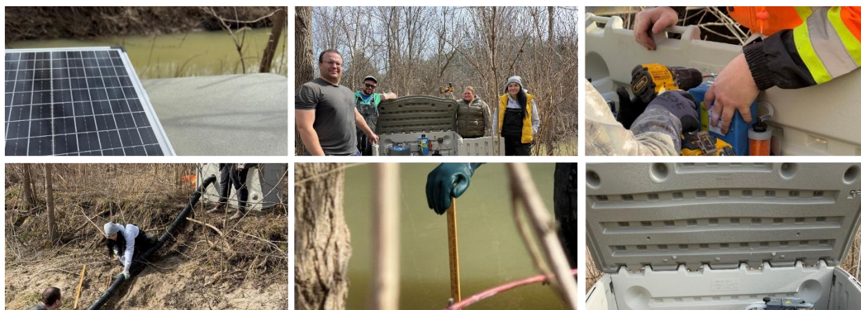
Figure 1. Photographs of the field crew installing ISCO 6712 autosampler at East Two Creeks.
