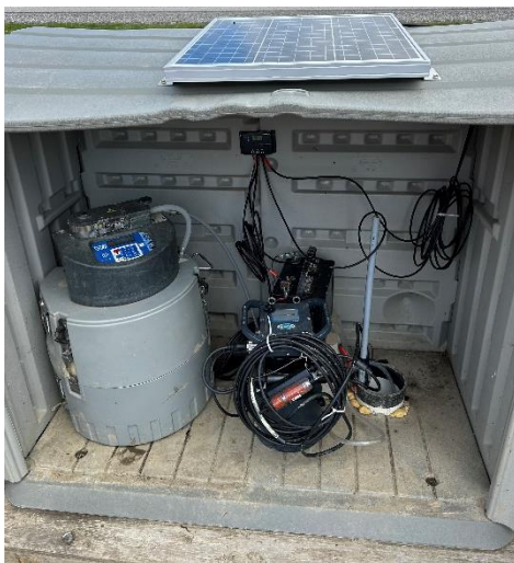
LTVCA Merlin edge of field site with new HACH AV9000 area-velocity equipment.
