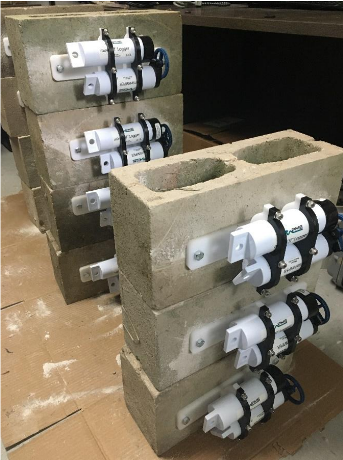
Figure 3: PME miniDOT Oxygen loggers for sampling dissolved oxygen and temperature conditions in aquatic environments.
