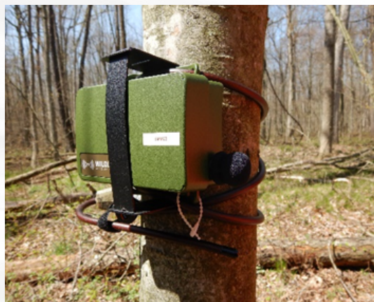
A Mini Song Meter installed at the Mosa Forest Conservation Area to detect the sounds of breeding birds and amphibians.
