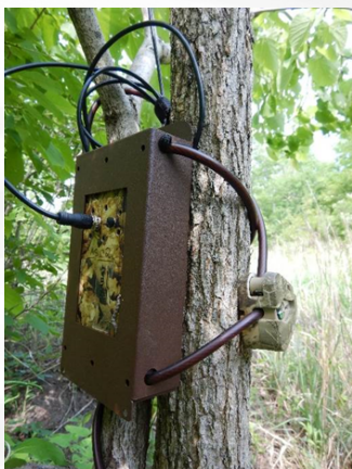
An Anabat Swift bat detector installed at the Mosa Forest Conservation Area.
