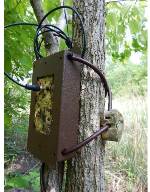
Figure 2: An Anabat Swift bat detector installed at the Mosa Forest Conservation Area.
