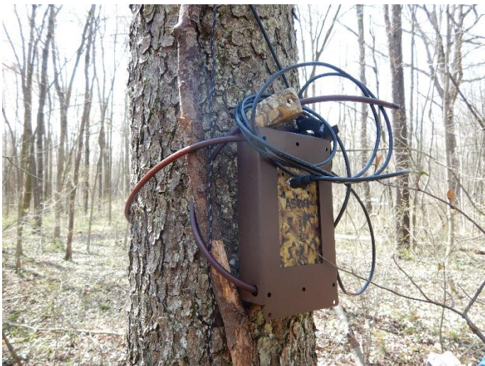
Figure 5: An Anabat Swift monitoring unit installed at the Mosa Forest Conservation Area to detect bats.
