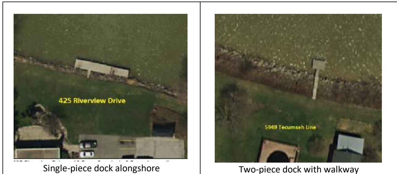
Figure 2.1: Sample Docks in the Lower Thames River (photos courtesy of V. Towsley, LTVCA)
