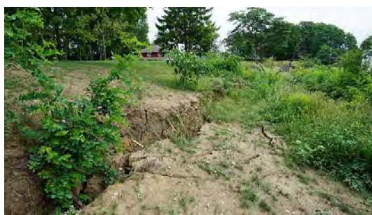
Figure 2.19 Formation of Tension Crack Along Bluff Crest
