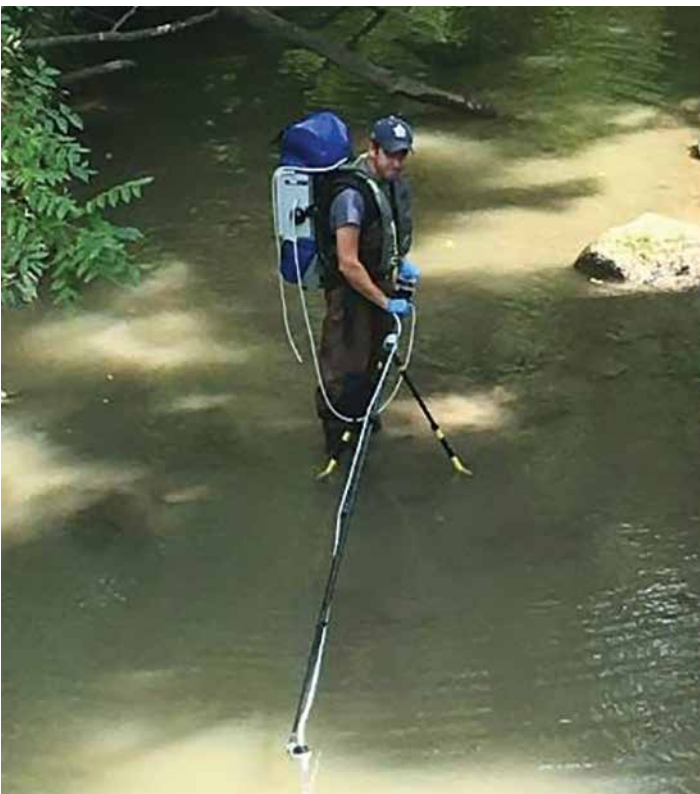
Daniel Nydam - Species at Risk Assistant uses an eDNA sampler. The sampler was purchased, four staff were trained in its use and sampling occurred in seven LTVCA subwatersheds to detect presence of fish and mussel SAR. Staff conducted seine netting of fish at three sample sites and collected mussel shells found at all sites to help verify SAR present.
