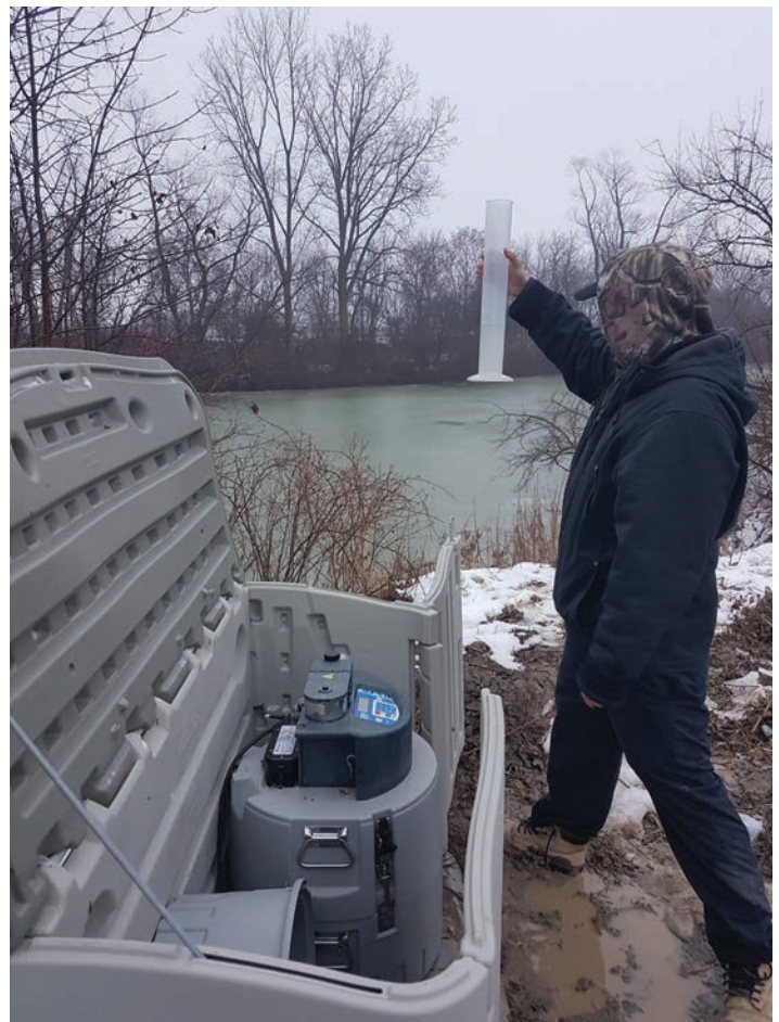
Austin Pratt calibrates the water volume from ISCO autosampler at one of three pump stations being monitored for the GLASI Jeanette's Creek PSP to see the effectiveness of BMPs in regards to water quality.
