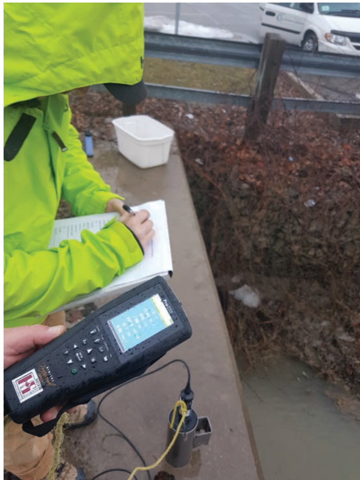
Staff take water samples at Indian Creek in Chatham, as well as using the YSI sonde to take in-field water quality readings such as pH, temperature, specific conductivity, dissolved oxygen and turbidity.
