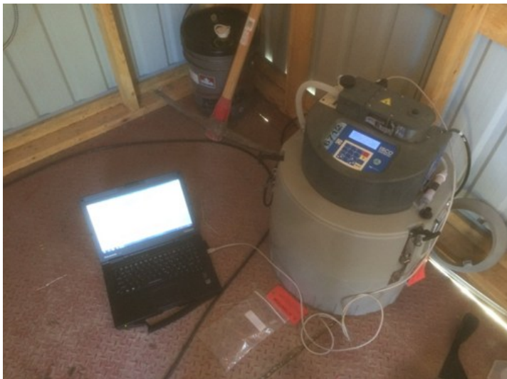
ISCO Water Quality Auto-Sampler at Boudreau Pump Station located in the Jeannettes Creek subwatershed
