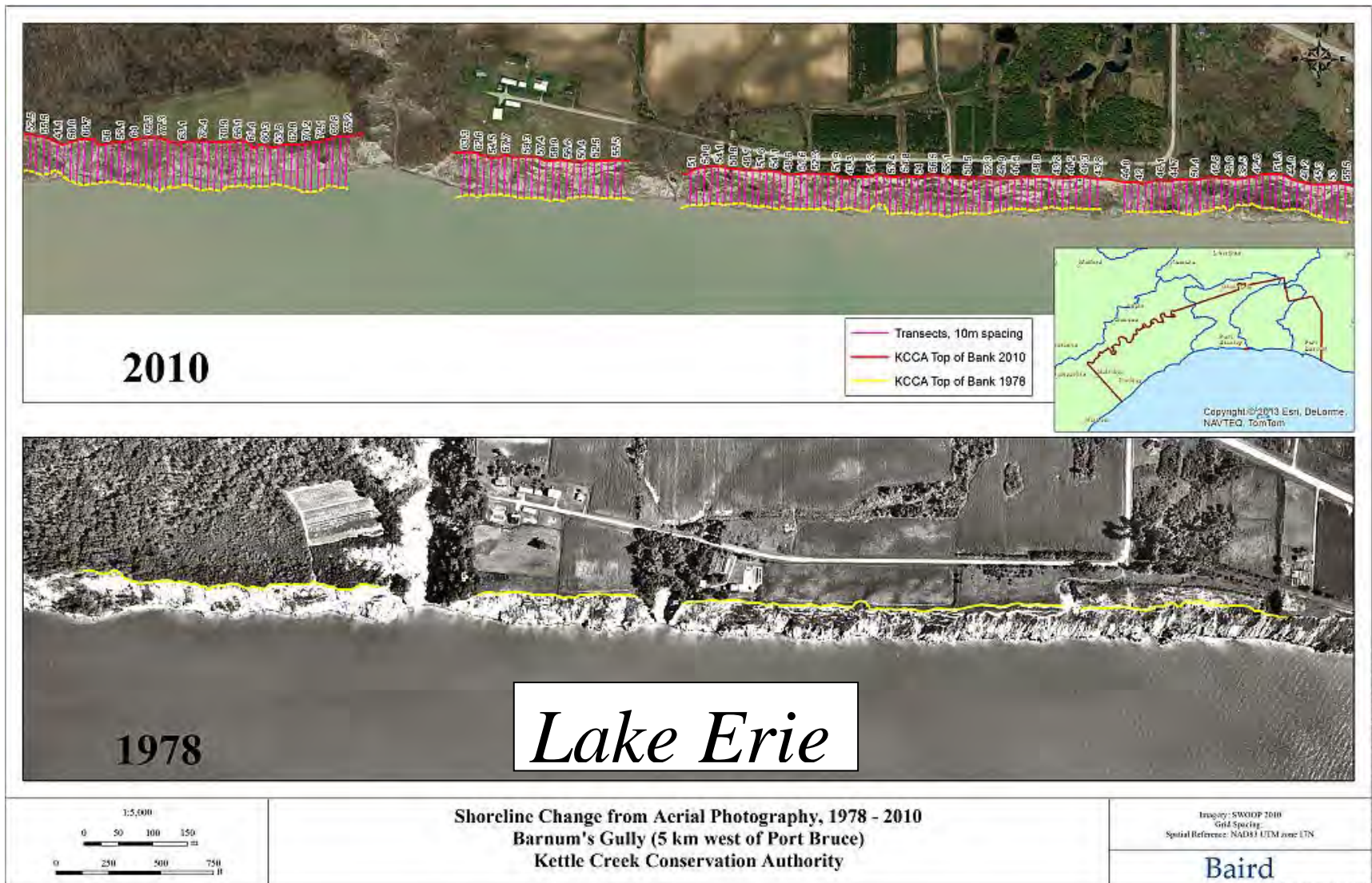
Figure 2.24 1978 to 2010 Erosion Measurements at Barnum's Gully, KCCA
