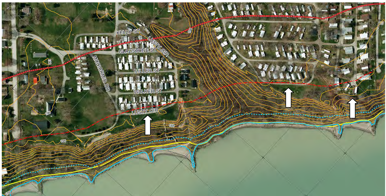
Figure 5.7 3:1 Stable Slope (red dash-dot line) and 100 Erosion Hazard Setback (red dashed line). White Arrows Identify Roads/Buildings in the Zone of Higher Risk
