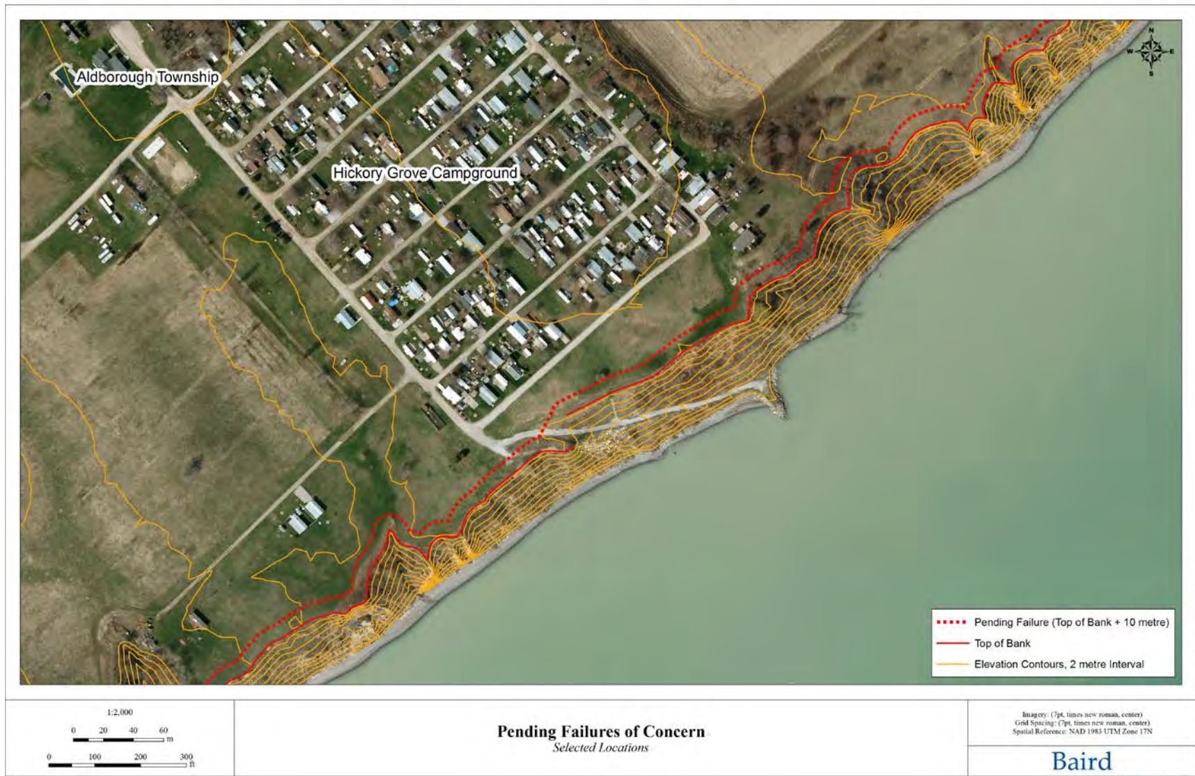
Figure 4.15 Zone of Pending Failure at Hickory Grove Campground, Municipality of West Elgin
