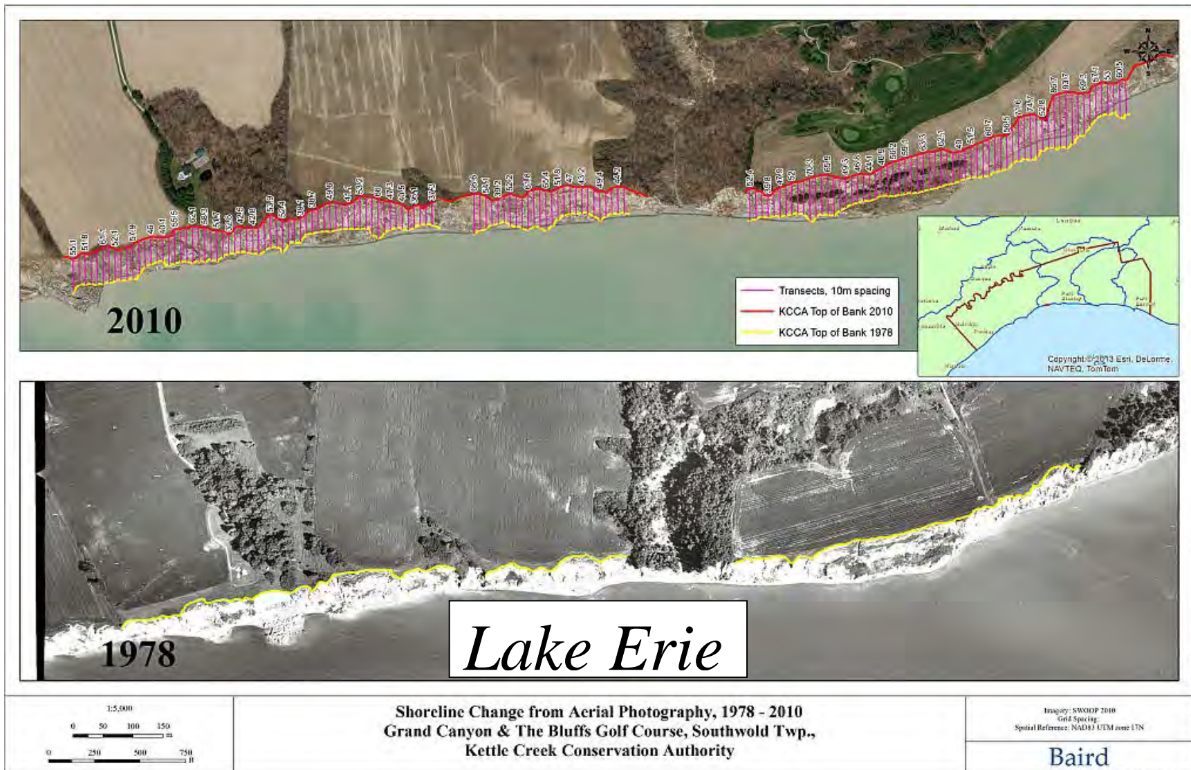
Figure 2.23 1978 to 2010 Erosion Measurements at Grand Canyon and the Bluffs Golf Course, KCCA
