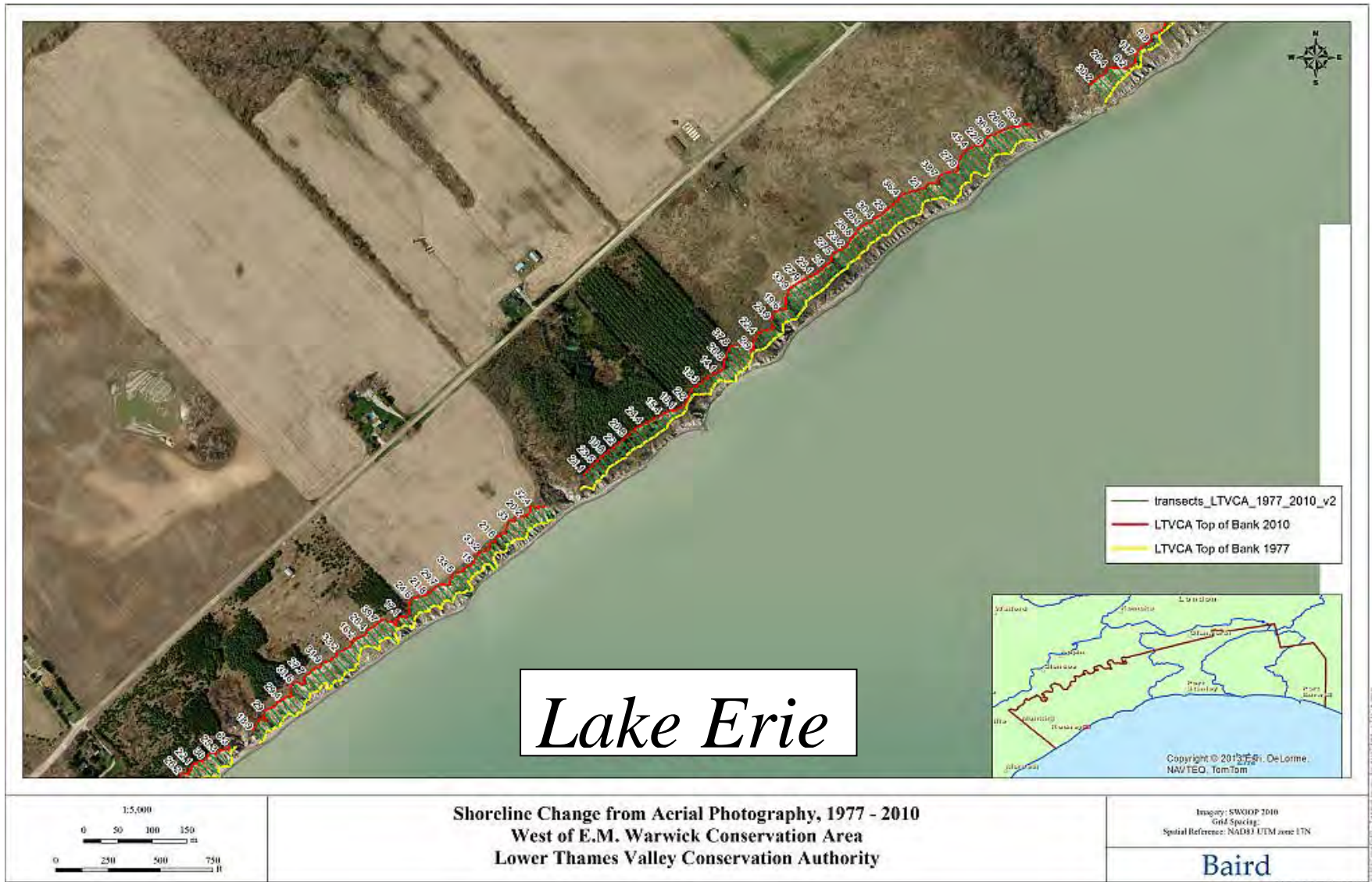
Figure 2.19 1977 to 2010 Erosion Measurements West of E.M. Warwick Conservation Area, LTVCA
